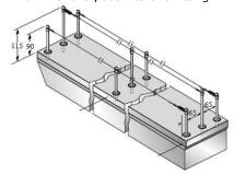
2.3.2 Steel, sheet metal, or concrete, stone or brick with no holes in substrate. Use stick on bases and silicone adhesive.
